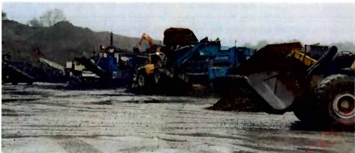
Fig. 2: Loading and operation of mobile crushing and screening plant on the quarry floor
